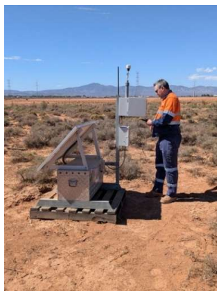
An Ecotech technician carrying out scheduled maintenance on a dust monitor.
